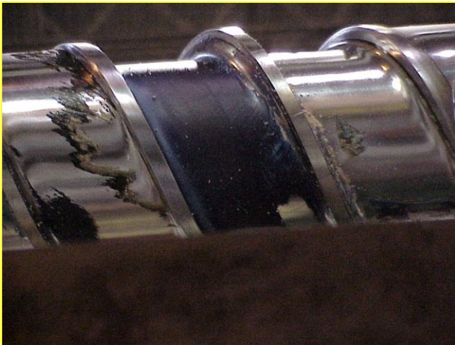
Customers' Screws Stained with Pigments
