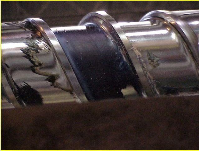
Customers' Screws Stained with Pigments
