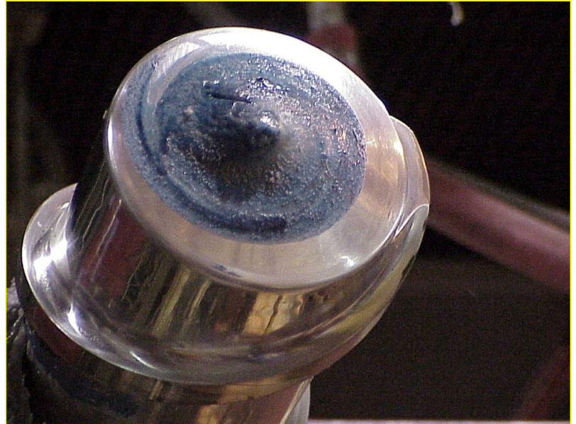
Customers' Screws Stained with Pigments
