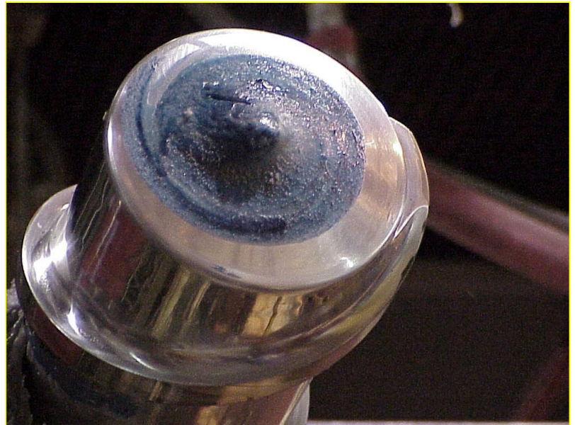
Customers' Screws Stained with Pigments
