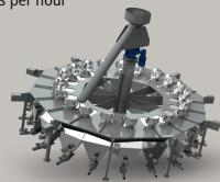
3 A dispensing manifold with a rotating arm and up to 50 buffer bins
