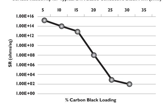
Surface Resistivity for Typical EVA Based Conductive Black Film (5mil)
